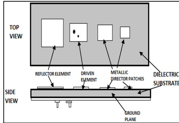
**Figure 1: Microstrip Yagi-Uda Configuration**
